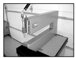
\*\*To protect from accidentally releasing the handle while working which could create an unwanted dimpled hole, a balanced (low force) return system is incorporated in the design. This solution provides protection while minimizing the resistive load on the operator.
